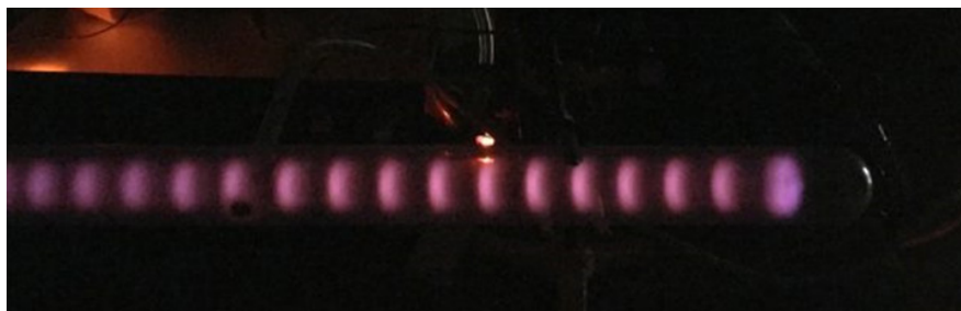
Figure 34: Positive column of a DC glow discharge.
